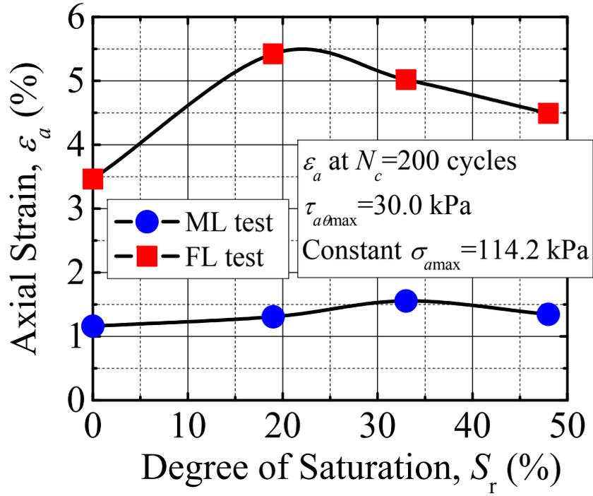
Cyclic plastic deformation under different loading conditions and  $S_r$
