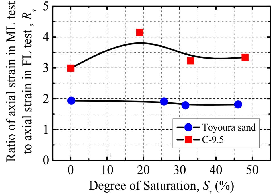
Cyclic plastic deformation under different loading conditions and  $S_r$
