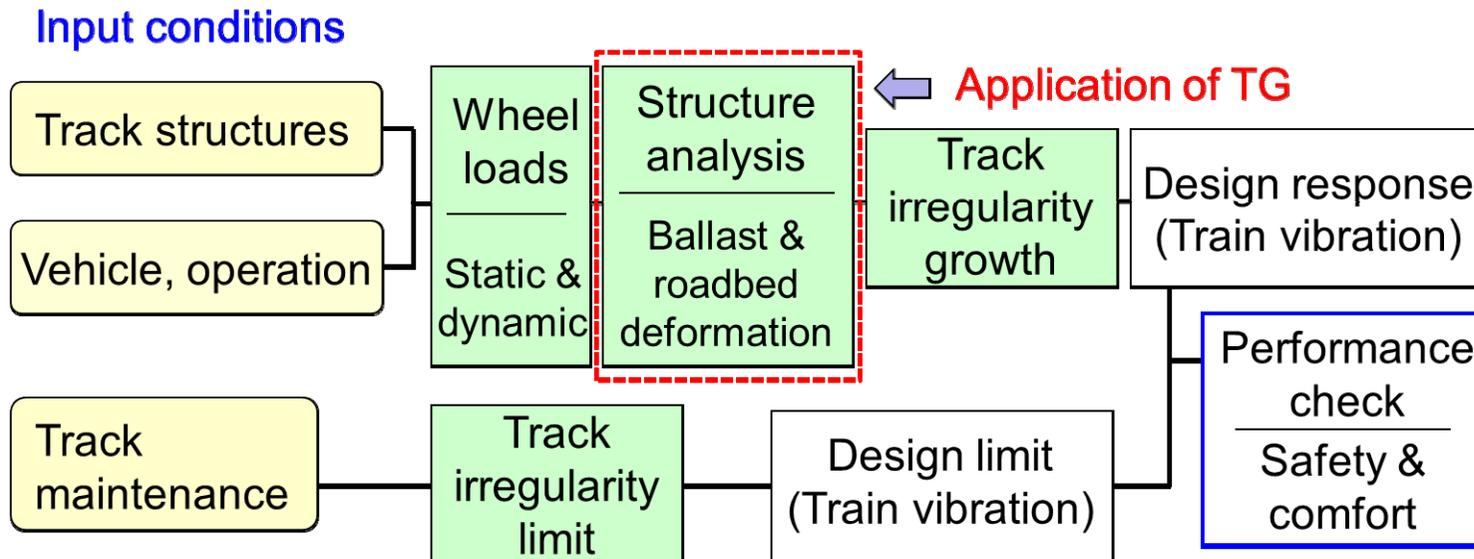
Flow of design procedures for ballasted track
