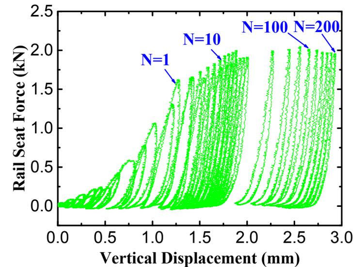
Moving wheel loads give a large residual settlement as compared with fixed-point cyclic loads.
